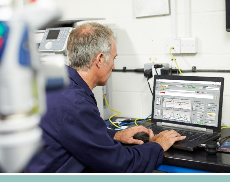
COMPUTERIZED MANAGEMENT OF ALL CONTROL PLANS, containing all the information required by quality standards, with search option by date of issue, plan type, department, article and product features. A list of the characteristic measurements associated with each drawing can be imported from files generated by the CAD / PLM / PDM systems.
